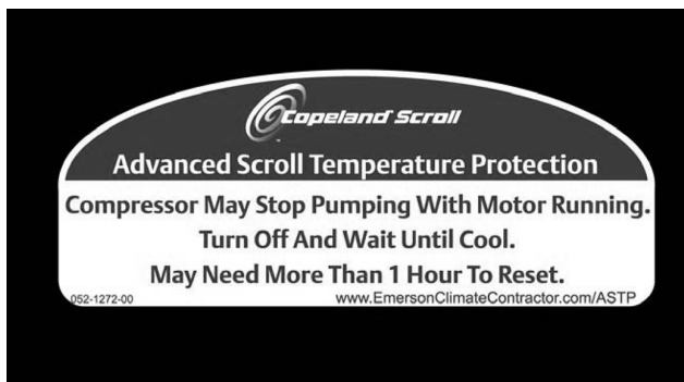
Fig. 15 — Advanced Scroll Temperature Protection Label
